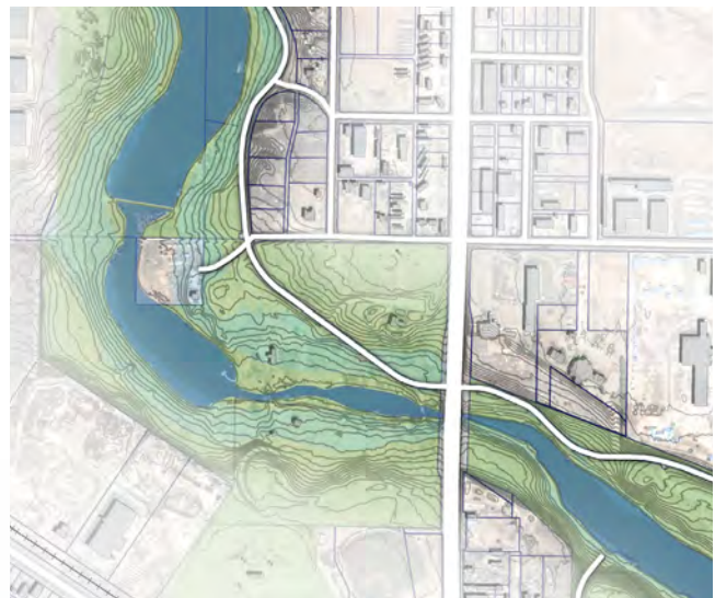
The above two-foot contour map of Hodges Park demonstrates the elevation changes surrounding the Canyon Lakes in the Yellow House Canyon compared to the relatively flat topography outside of the Canyon.
