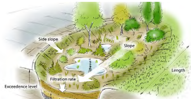
Graphic depicting a micro-detention pond Source: Innovye Resource Center
