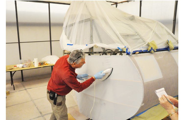
Heat is carefully applied to shrink the polyester fabric taut to the cockpit structure.
