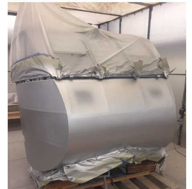
Silver-impregnated dope over clear base layers protects the fabric from ultraviolet light.
